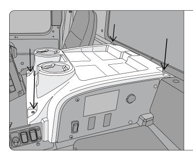
**Step 8:** Clean up all wiring using cable ties. Complete an installation check for the GO device, then reinstall the center console cover.
