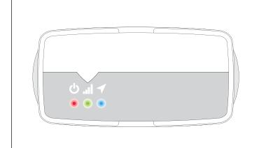
**Step 10:** Start the engine, leaving it to idle. All three LED's will flash red briefly - wait until you see all three LED's: Red (Power), Green (GSM) and Blue (GPS). These tell you the unit has connected successfully.
