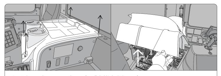
Step 1: Remove the center console cover (usually held in by T25 screws).
