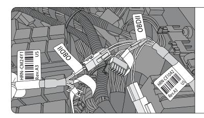
**Step 5:** Take the HRN-CM24Y1 and connect the 6-pin white Molex connector labeled OBD2 with the 6-pin white connector labeled OBD2 from the HRN-CE10A2.
