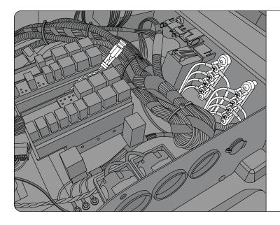
**Step 2:** Locate the power bus bar and the twisted yellow and green J1939 lines inside the center console area.
