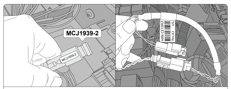
**Step 6:** Remove the terminating resistor from the green and yellow twisted pair connector labeled MCJ1939-2, then plug it into the mating end of the HRN-CE10A2. Connect the HRN-CE10A2 to where the terminating resistor was removed from MCJ1939-2.
