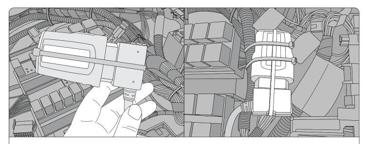
**Step 7:** Connect the HRN-CM24Y1 to the GO device and secure the connection with a cable tie. Use two additional cable ties to secure the GO device inside the center console.
