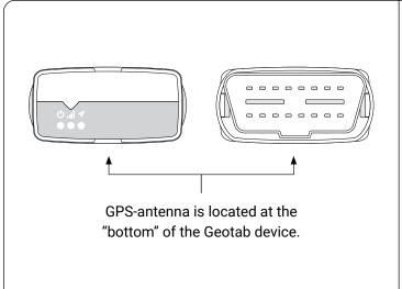
**Step 7:** GPS-antenna is located at the "bottom" of the Geotab device. Ensure this side is facing away from any metal surface when securing the device into the vehicle.
